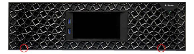
After removing the two screws, pull the fascia forwards and straight off the unit. It is retained by four push-fit fasteners. If the fascia sides are inaccessible, plastic hooks are provided to pull the fascia off (see Installation  $^{(5)}$ ).
