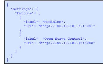
Will introduce new buttons to these addresses on the bottom of the Settings menu:
